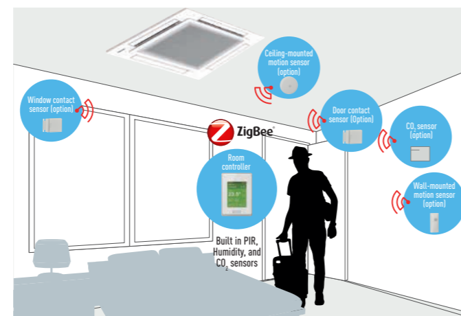
Batteries last for up to five years and are easy to install and replace.
